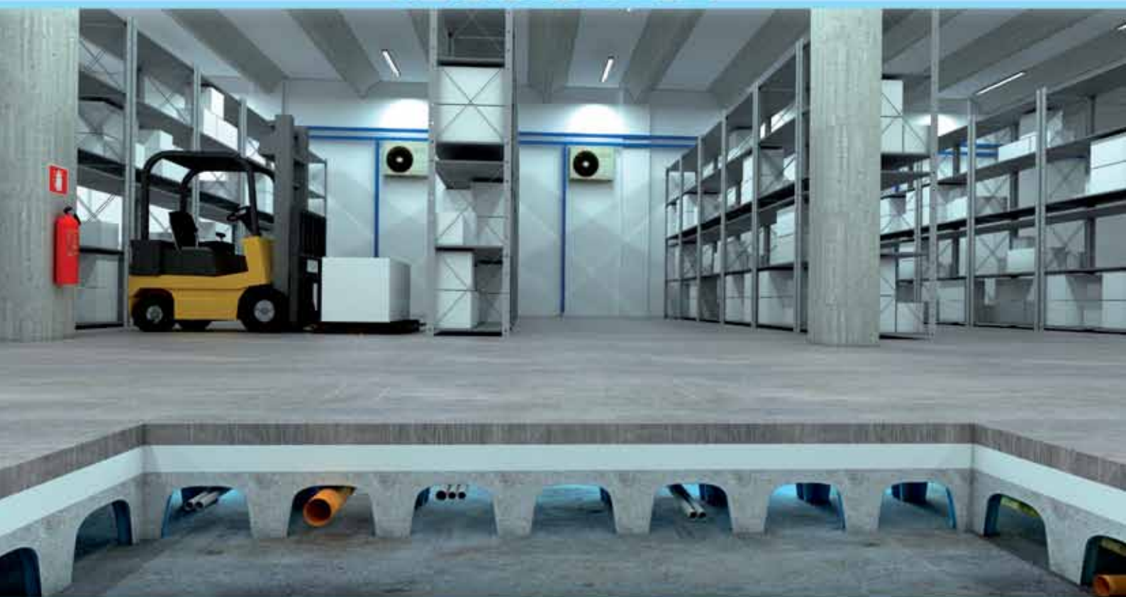
Ventilation system for negative refrigeration cells
